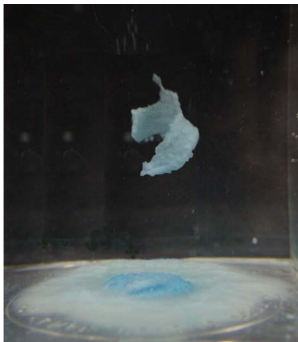
Figure 1 The Chemical Canon. The flake moves above the rest of the pellet. 0.10M \text{Na}_2\text{CO}_3 . Pellet: \text{CuSO}_4 \times 5\text{H}_2\text{O} .
